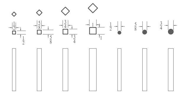
Rail picket samples: They are available as shown and as solid shapes, they can be vertical or horizontal and the square shapes can be turned 45° to create a diamond effect. All square shapes are available as hammered or twisted.
